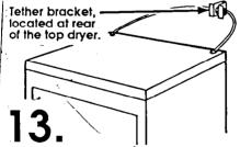
Attach both ends of tether located at the rear of the top dryer to a secured 2x4.
